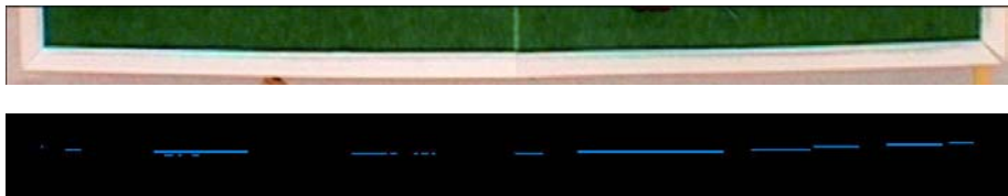
Blue color regions appear near a field boundary by the characteristics of frame grabber. The color segmentation algorithm detects them as the candidate segments
